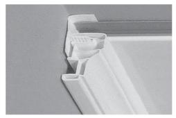
Fit wall boards flush with ceiling, \*Spot drill through mounting strip and wall board at regular intervals. Drill out the wall and fit wall plugs flush with the surface of the wall board. Fix the mounting strip using flat head screws. Fit the ceiling boards and finish by clipping the front face of the cornice into place.
